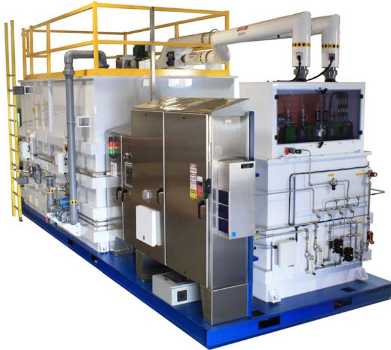
Shown: PDP-200-2-SC-G-B-T-AX-4-N4XS-LR-LK-FL-DL. 200 gpm system, 2 reaction stages, acid and caustic addition, chemical day tanks, 460 VAC control panel with Allen Bradley CompactLogix PLC and 10" PanelView Plus HMI
