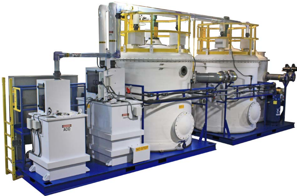
Shown: PDP-400-2-SC-G-B-T-AX-4-N4-LR-LK-FL-DL. 400 gpm system, 2 reaction stages, acid and caustic addition, chemical day tanks, 460 VAC control panel with Allen Bradley CompactLogix PLC and 10" PanelView Plus HMI
