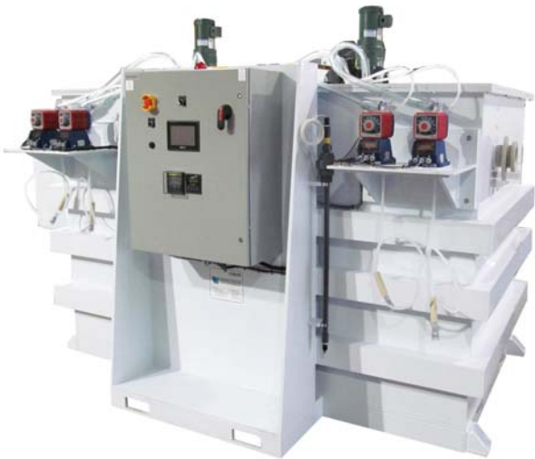
Shown: PDP-50-2-SC-G-B-M-IM-1-N4-LR. 50 gpm system, 2 reaction stages, acid and caustic addition, chemical metering pump shelf, 115 VAC IDEC with Maple HMI control panel.
