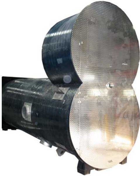
Shown: 2500 gallon triplex pump lift station with side inlets, CPVC piping, and multiple hatches for equipment and valve access.
