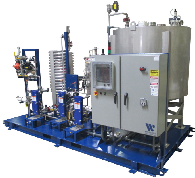
Shown: BDC-DUO-10-90-90-SH-CW-AX-4-N4-DL. 10 gpm system, 90 °C, 90 second hold time, steam heat exchanger, chilled water heat exchanger, pH neutralization (separate skid—not pictured), 460 VAC NEMA 4 control panel with Allen Bradley CompactLogix PLC and 10" Maple HMI.
