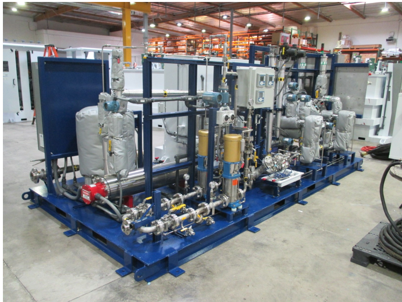
Shown: BDC-DUO-8-140-60-EH-CW-AX-4-N4XS-ASME-DL. 8 gpm system, 140 °C, 60 second hold time, electric heater, chilled water heat exchanger, pH neutralization, includes insulation, 460 VAC NEMA 4X control panel with Allen Bradley CompactLogix PLC and 10" Maple HMI.
