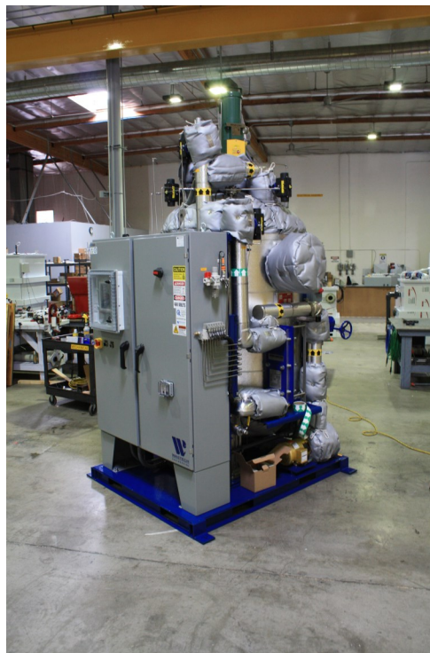
Shown: BDB-265-121-60-SI-CW-AX-4-N4-DL-IN. 265 gallon inactivation tank, 121 °C, 60 minute hold time, direct steam injection to tank, chilled water heat exchanger, includes insulation, 460 VAC NEMA 4 control panel with Allen Bradley CompactLogix PLC and 10"
