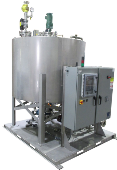
Shown: BDB-500-93-30-SI-CW-AX-4-N4-HT-FL-DL. 500 gallon inactivation tank, 1000 gallon holding tank, 93 °C, 30 minute hold time, direct steam injection to tank, chilled water heat exchanger, 460 VAC NEMA 4 control panel with Allen Bradley CompactLogix PLC and 10" Maple HMI.
